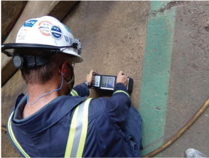
Figure 3. UST survey being performed as part of a foundation assessment at a chemical plant.
