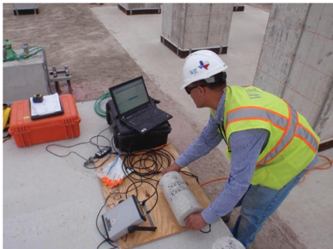
Figure 5. UPV testing on concrete cylinders which were used for a baseline velocity as part of an evaluation of columns on a compressor foundation.
