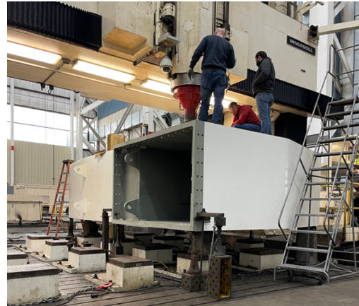
Machining a counterweight girder
